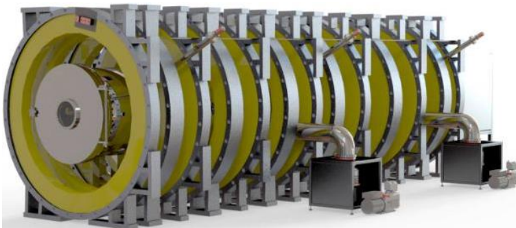
Conceptual drawing of the SPEKTRE device. The main vacuum vessel, 6 m long and 90 cm in diameter, houses a plasma confined by 13 copper coils (in yellow).
