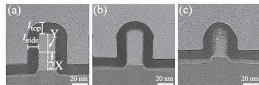
Fig. 2. TEM images of TiO<sub>2</sub> films deposited on a-C patterned substrates<sup>5</sup>. The mean ion energy,  $\langle \varepsilon_i \rangle$ , in CCRF discharges is (a) 23 eV, (b) 73 eV and (c) 133 eV, respectively.
