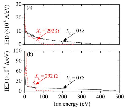
Fig. 1. Ion energy distribution (IED) in CCRF discharges<sup>4</sup>. IEDs are modified via the impedance controller connected with the wafer stage. The impedance at the wafer stage is controlled by the reactance of the controller,  $X_L$ . (a) and (b) correspond to RF power of 300 W and 1000 W, respectively.
