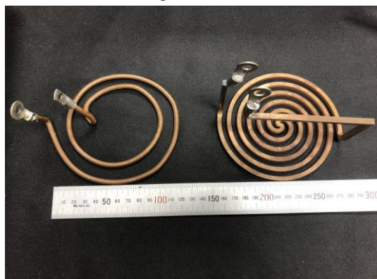
Fig. 1 A photograph of spiral antennas employed to the presented experiments.
