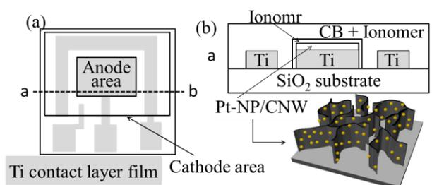
Fig. 2 (a) Top view and (b) cross-sectional view of glucose fuel cell fabricated in this study
