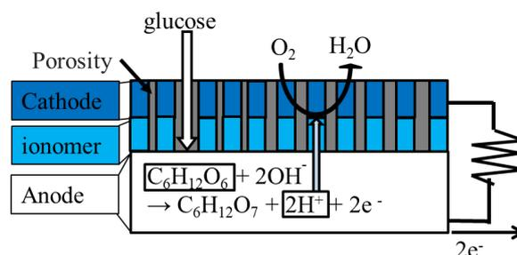
Fig. 1 Schematic illustration of glucose fuel cell
