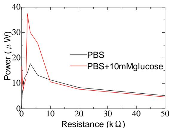
Fig. 3 Measured output resistance-power characteristics
