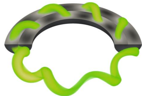
Helical self-organization in Reversed Field Pinch. Pictorial view of plasma displacement obtained in experimental-like 3D nonlinear MHD numerical modelling.
