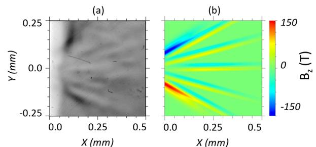
Figure 1. (a) Proton image of a laser-irradiated foam target, showing the development of e.m. fields and filamentation inside the target. (b) Magnetic field distribution reconstructed via comparison with particle tracing simulations.
