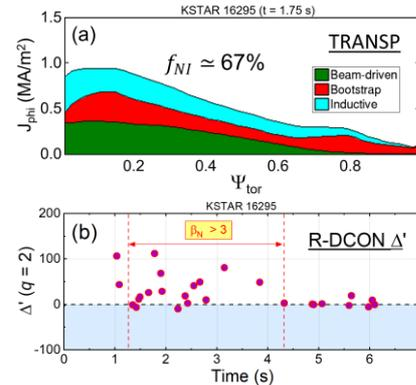
Figure 2. For high  $\beta_N$  plasma, (a) non-inductive current profiles from TRANSP and (b) resistive DCON computed  $\Delta'$ .
