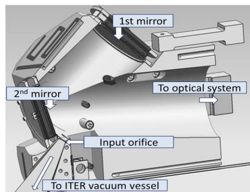
Figure 1. The FEOT of the UWAVS, with positions of the mirrors, input orifice open to the vacuum vessel and the direction toward the rest of the optical system. The positions of the RF feeds are not shown.
