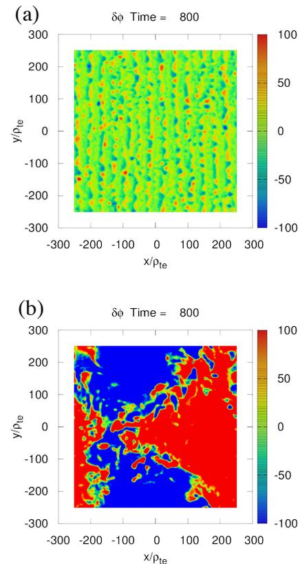
Figure 2. Contours of the normalized electrostatic potential fluctuations with (a) adiabatic ion, and (b) kinetic ion.
