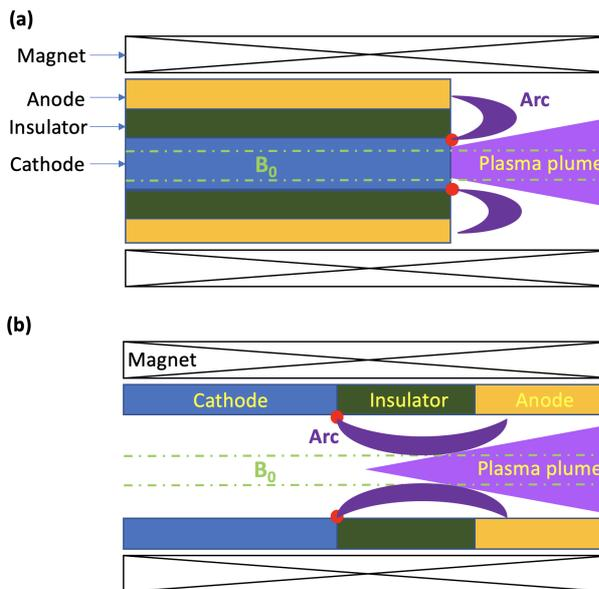
Fig 1. Schematics of typical magnetically enhanced vacuum arc thruster (MEVAT): (a) coaxial-type, (b) ring-type.
