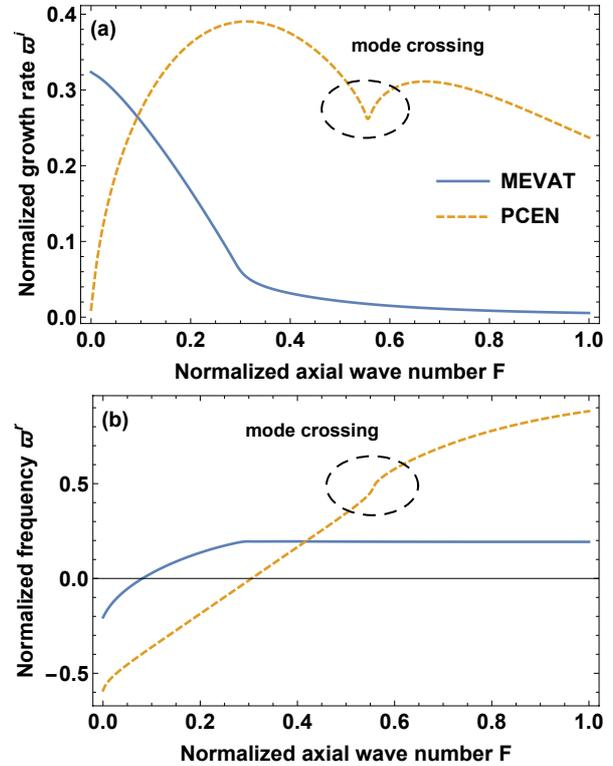
Fig. 2 Dispersion curves for MEVAT (solid line) and PCEN (dashed line), generated based on the conditions shown in Table I: (a) normalized growth rate  $\omega^i$ ; (b) normalized frequency  $\omega^r$ . (vs normalized axial wavenumber  $F = k_\zeta/\sqrt{\delta}$ )
