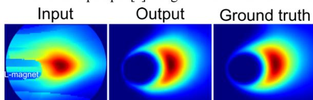
Fig. 1. Sample reconstructions produced by the network, with the line-integrated image (Input, left), reconstructed local emissivity (Output, middle), and target image (Ground truth, right).
