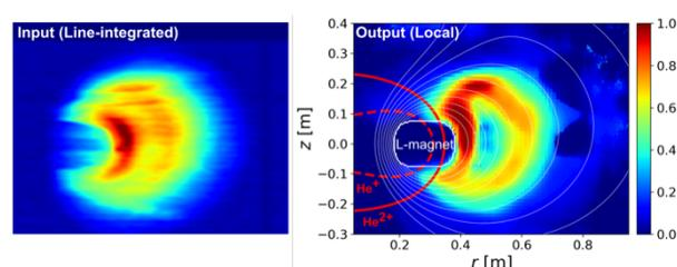
Fig. 2. Line-integrated emission intensity of CIS (left) and reconstructed local intensity profile (right) with ICRF. The ion cyclotron layers for He<sup>2+</sup> and He<sup>+</sup> are depicted.
