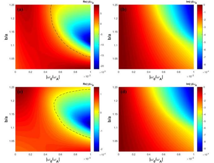
**Fig. 1.** The (a,c) growth rate, and (b,d) real frequency, of the  $n=1$  PRRWM with varying wall radius  $b/a$  and the plasma toroidal rotation frequency  $\omega_0$  (normalized by the Alfvén frequency  $\omega_A$ ), as calculated by the analytic model. Compared are the case without (a,b) and with (c,d) thermal transport terms (TTT). Dashed lines indicate marginal stability of the mode.
