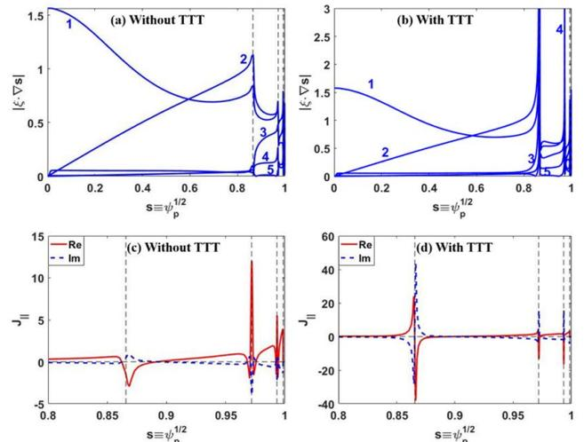
**Fig. 2.** Radial profiles of the poloidal Fourier harmonics for (a,b) the radial displacement, and (c,d) the  $m/n=2/1$  perturbed parallel plasma current density, associated with the  $n=1$  RPRWM computed by MARS-F. Solid (dashed) curve in (c,d) denotes the real (imaginary) part of the perturbed parallel current. Compared are the eigenmode structures between the cases without (a,c) with (b,d) TTT.
