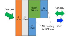
Fig. 1 Schematic setup in laser shock experiments.
