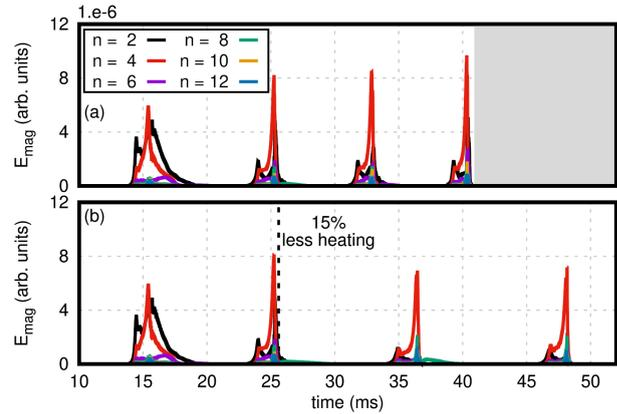
Figure 1: Magnetic energies of the non-axisymmetric perturbations of the simulated type-I ELMs. Reducing the heating power [after  $\sim 26$  ms in panel (b)] shows a decrease in  $f_{\text{ELM}}$ , as expected for type-I ELMs.
