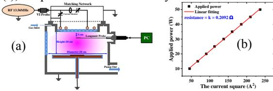
Fig. 1, the schematic diagram of the experimental setup (a) and the measured equivalent resistance (b).
