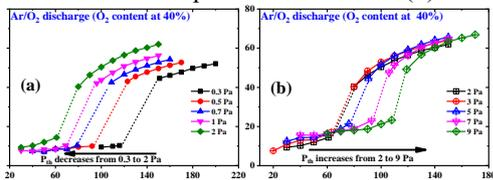
Fig. 2, the  $\eta$  against the applied power during the E to H mode transition at the pressure from (a) 0.3 to 2 Pa and (b) 2 to 9 Pa for Ar/O<sub>2</sub> discharge and the O<sub>2</sub> content is 40%, respectively.
