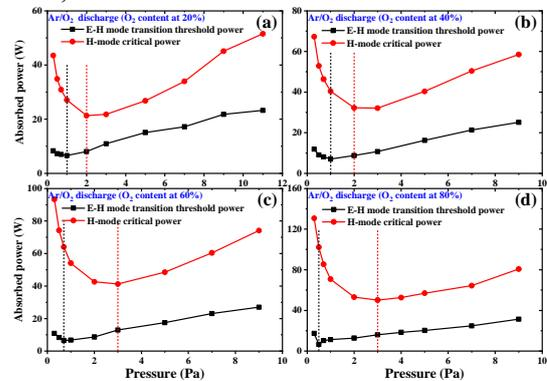
Fig. 4, the transition threshold power in absorbed power against the pressure for Ar/O<sub>2</sub> discharge in different O<sub>2</sub> content at (a) 20%, (b) 40%, (c) 60% and (d) 80%, respectively.
