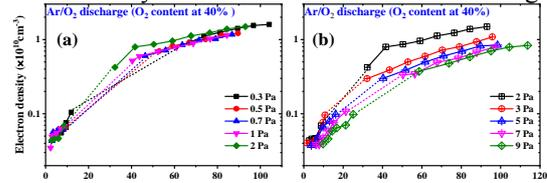
Fig. 3, The electron density against the absorbed power at the pressure from (a) 0.3 to 2 Pa and (b) 2 to 9 Pa for Ar/O<sub>2</sub> discharge and the O<sub>2</sub> content is 40%, respectively.
