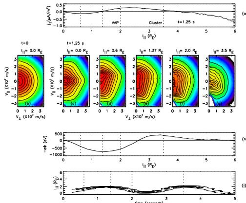
**Figure 1:** (a) Parallel current density as a function of distance along the field line. (b) Initial Maxwellian distribution function at  $t = 0$ . (c)–(g) Electron distribution functions at  $t = 1.25$  s and the indicated values of  $l_{||}$ . (h) Effective potential at  $t = 1.25$  s. (i) Evolution of an ensemble of trapped electrons taken from core of distribution evident in panel f (from [7]).
