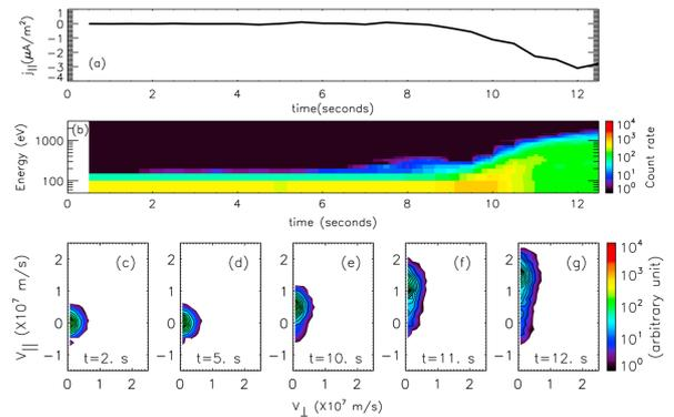
**Figure 2:** (a) Parallel current above the ionospheric boundary as a function of time. (b) Electron energy spectrogram above the ionospheric boundary. (c)–(g) Corresponding electron distribution functions at the indicated times (from [8]).
