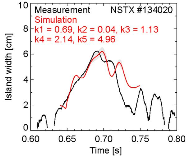
Fig. 3. Comparison of measured (black) and simulated (red) island width time evolution. The shaded area indicates the error bar of the simulation. Modified Rutherford equation coefficients  $k_1 - k_5$  are also shown.
