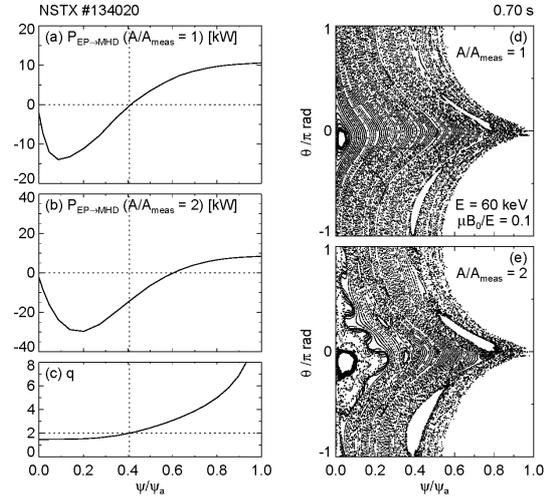
Fig. 2. Profiles of power transfer from energetic particle to modes for the case where mode amplitude is (a) the same, and (b) twice as measured mode amplitude, and (c) safety factor. Poincaré plots for the case where mode amplitude is (d) the same, and (e) twice as measured mode amplitude.
