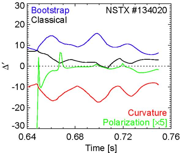
Fig. 1. Comparison of classical (black), bootstrap current (blue), polarization current (green) and curvature (red) effect on NTM stability. Without the energetic particle contribution, the polarization current effect should be suppressed to be zero for the simulation to match the measurement of island width.
