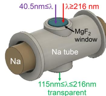
FIG.1 A schematic diagram of the sodium tube installed MgF<sub>2</sub> windows for direct Na observation.
