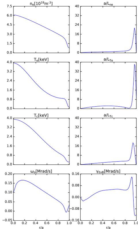
**Fig. 1** Profile analysis results of KSTAR H-mode discharge (shot 25690, time=5720ms). Right three figures show inverse gradient scale length of quantity normalized by minor radius,  $a/L_x$ .  $\omega_o$  and  $\gamma_{ExB}$  denote rotation frequency and ExB shearing rate, respectively. Their definition can be found in [3]
