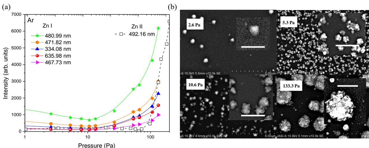
Figure 1 (a) Intensity of Zn species from the optical emission at different pressure for ablation in Ar. (b) The deposited nanostructures increases in size as Ar pressure increases. The scale bar of the inset is 1 μm.
