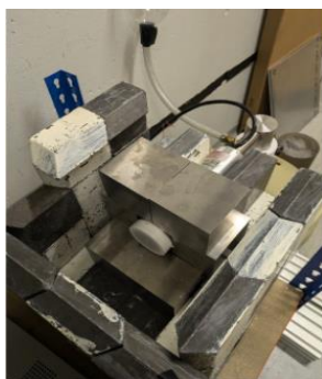
Figure 1. The passive background suppression system for the HPGe detector surrounded by tungsten and lead bricks
