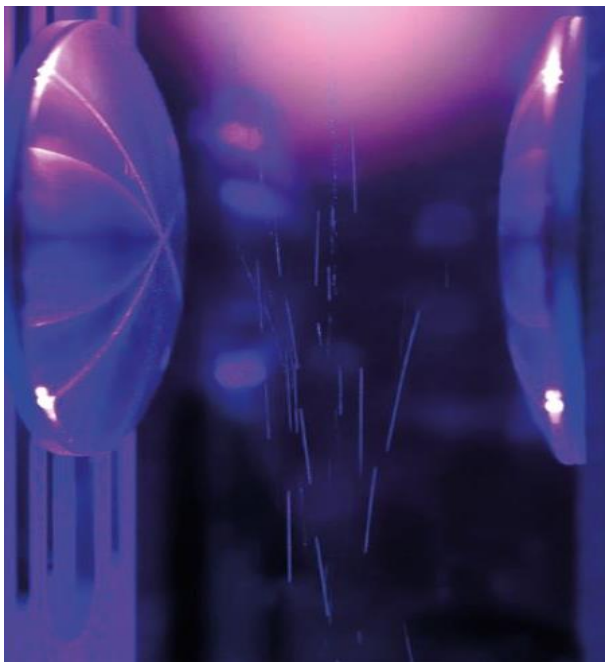
Figure 1: Two deflecting electrodes create a horizontal electric field in the afterglow region of an inductively coupled radiofrequency plasma. This field influences the trajectories of falling microparticles, which were previously electrically charged by the plasma.
