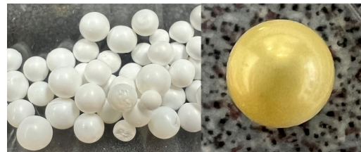
Figure 1. (LEFT) DCPD/NB foam shells, dry, with nominal foam density of 25 \text{ mg/cm}^3 , diameters 3-4 mm. (Right) DCPD/NB foam shell overcoated with \sim 6 \text{ }\mu\text{m} of GDP (glow discharge polymer).
